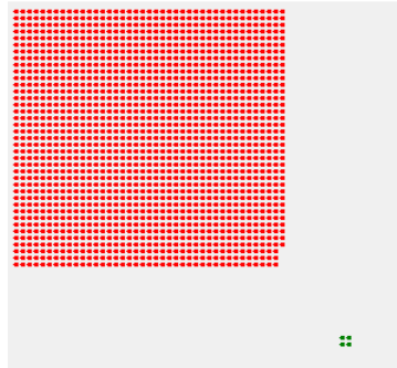
Figure 1: The initial position of the robots and the seed robots. The seed robots are green, the other robots are colored red.
