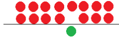
Figure 12: Robot jumps over hole in structure. The red circles are robots that have already arrived at their final location, the green circle is the robot currently edge-following and the black line indicates the border of the global map.
